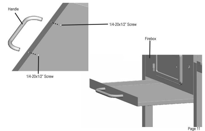
Attach Lid Handle and Handle Seats to the Lid using (2) 1/4-20x1/2" Screws.
